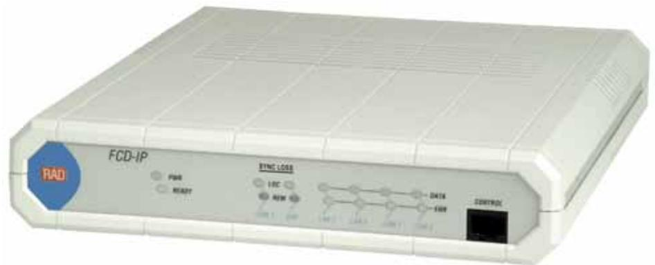
Integrated access device providing bundled services over E1/T1 access lines
