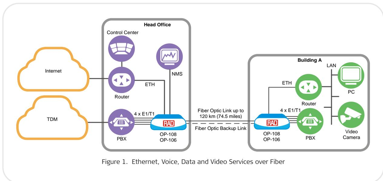
Figure 1. Ethernet, Voice, Data and Video Services over Fiber
