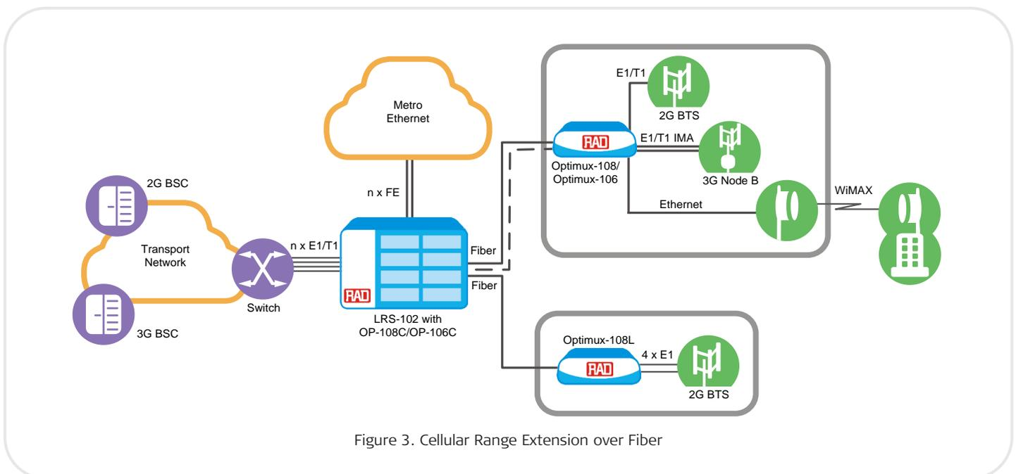
Figure 3. Cellular Range Extension over Fiber
